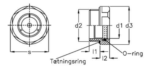
$\begin{array}{lll} d1 & = 18 \\ d2 & = G3/4 \\ d3 & = 32 \\ I1 & = 9.0 \\ I2 & = 8.0 \\ Max \ pressure & = - \\ Max \ vacuum \ mbar = - \\ s & = 30 \\ \end{array}$
